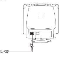
3. Connect the computer end of the D-SUB cable to the 15-pin output connector on the video board of your computer.
